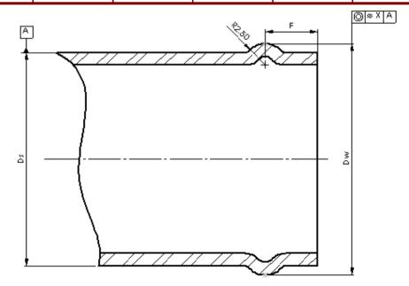
This tooling list has been generated as a design aid for customers wishing to utilise our standard hose bead tooling. These sizes are based on the hose bead specification in DIN 3021-3
